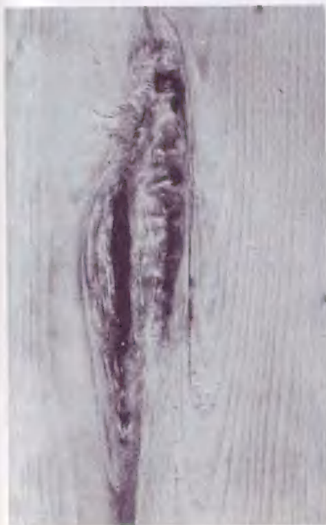
Pockets: Caused by damage to the cambial (tree growth) layer, repaired by the tree with bark or pitch.
